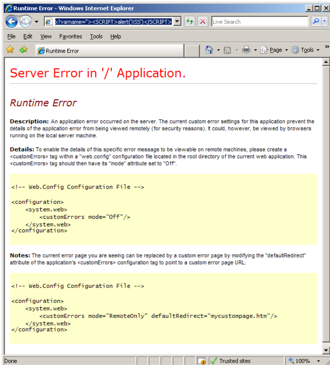
Figure 1 Default error page returned when submitting the malicious XSS payload to a remote server
