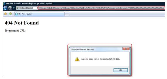
Figure 1 Exploiting the 404 error page XSS on Internet Explorer 7
