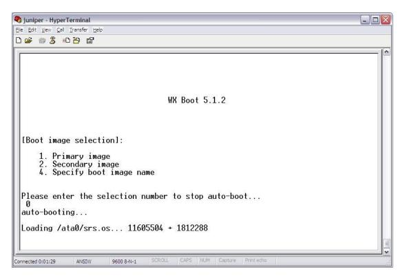
ProCheckUp found that by pressing the 5 key during boot up, caused a VxWorks boot menu to
