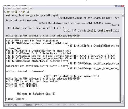
By pressing the reset button and powering on, an additional bootloader shell is sometimes displayed which allows new firmware to be uploaded to the device.
