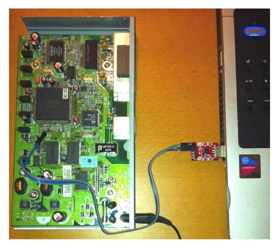
Version 5.0.94 boots into an interactive Linux shell, with later versions requiring authentication to gain access.
